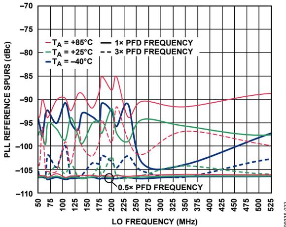
Figure 22. PLL Reference Spurs vs. LO Frequency
