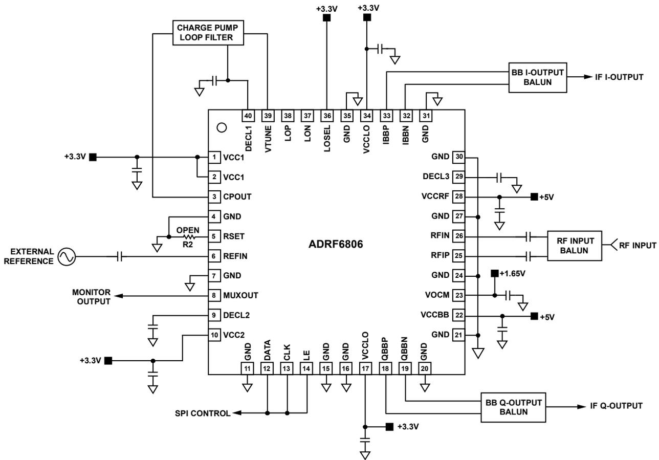
Figure 41. Basic Connections
