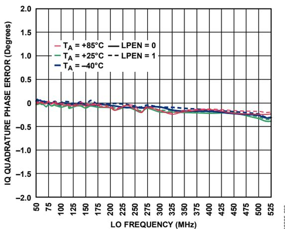
Figure 9. IQ Quadrature Phase Error vs. LO Frequency
