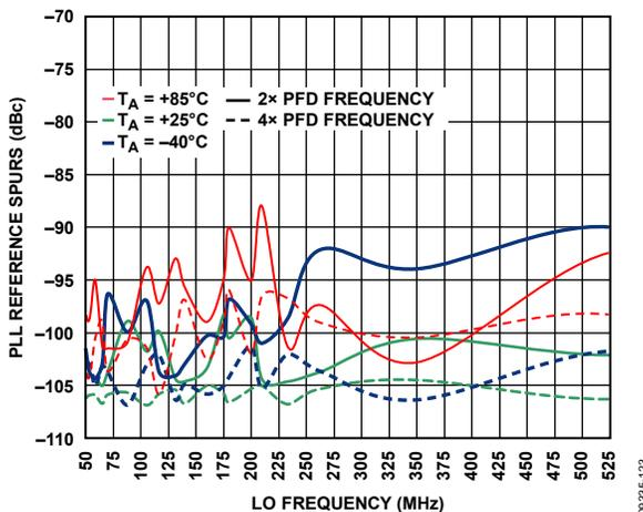
Figure 23. PLL Reference Spurs vs. LO Frequency
