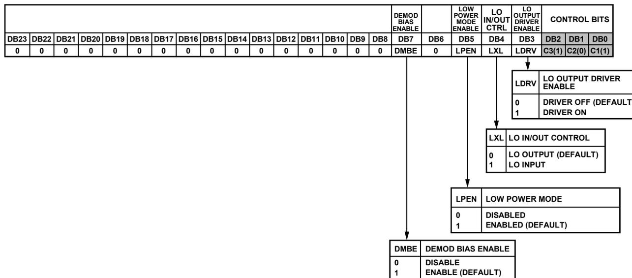
Figure 38. LO Path and Demodulator Control Register (R5)
