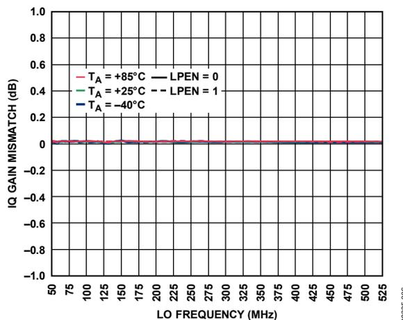
Figure 6. IQ Gain Mismatch vs. LO Frequency
